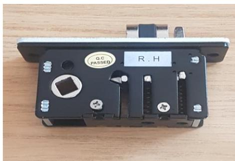
Remove the two coil springs.
