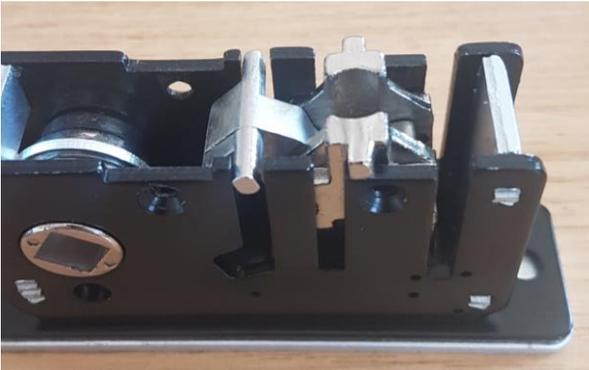
Reinsert the anti-thrust pin and the latch bolt that as shown. Place the springs back in place where they were previously found, replace the back plate and reinsert the screws as needed.
