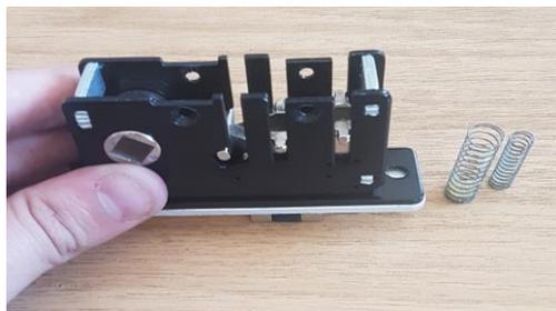
Prise the back plate off, using a flat headed screwdriver.
