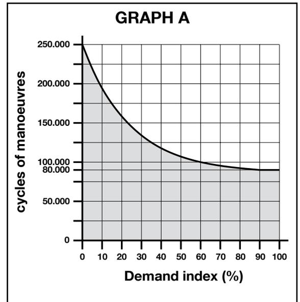
Example of calculation of durability of a Toona series 5 gear motor (refer to Table 2 and Graph A):
