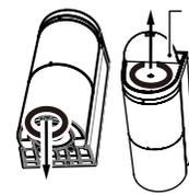
The rubber lid is difficult to reattach if it is detached completely. Flip it up to reach the screw.
