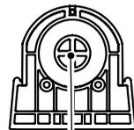
Break the knockout (wiring on conduit pipes)
