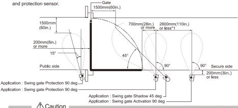
When 45 degree setting is set, it may not detect vehicles moving away from the sensor because it is
