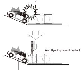
After the sensor is not detected, increase the sensitivity for the set time, Make it easier to detect vehicles that are moving backwards.
