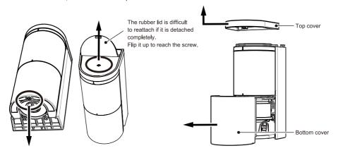
[2] Detach the sensor unit by lifting it.
