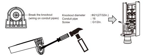
[3] When running a wire from a pole, cut the terminal cover with nippers by referring to the wiring holes on page 13, and put wires through the sensor housing.
