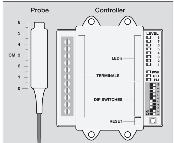
The MD102C is a control unit which enables configuration and testing of the MD102. DIP switches are used for configuration and LED's are used for visual indications of the operation of the probe. A relay output switches ON when a vehicle is detected.
