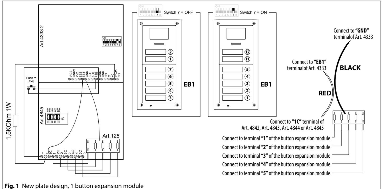
**Fig. 1** New plate design, 1 button expansion module
