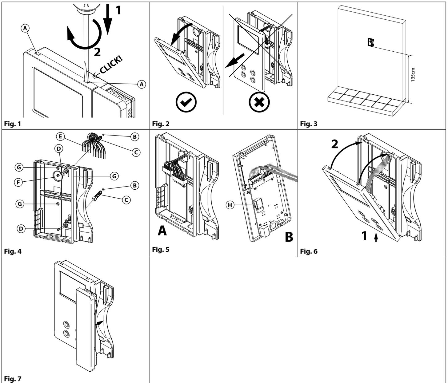
1. In order to install the videophone, it is necessary to remove the cover, which contains all the electronics, from the base: firstly disconnect the handset from the videophone (by removing its plug from the videophone) then insert a 5.5mm flat screw driver into the clip (A) then rotate clockwise until you listen a "CLICK!". Repeat the same operation with the other clip as shown in Fig. 1.
