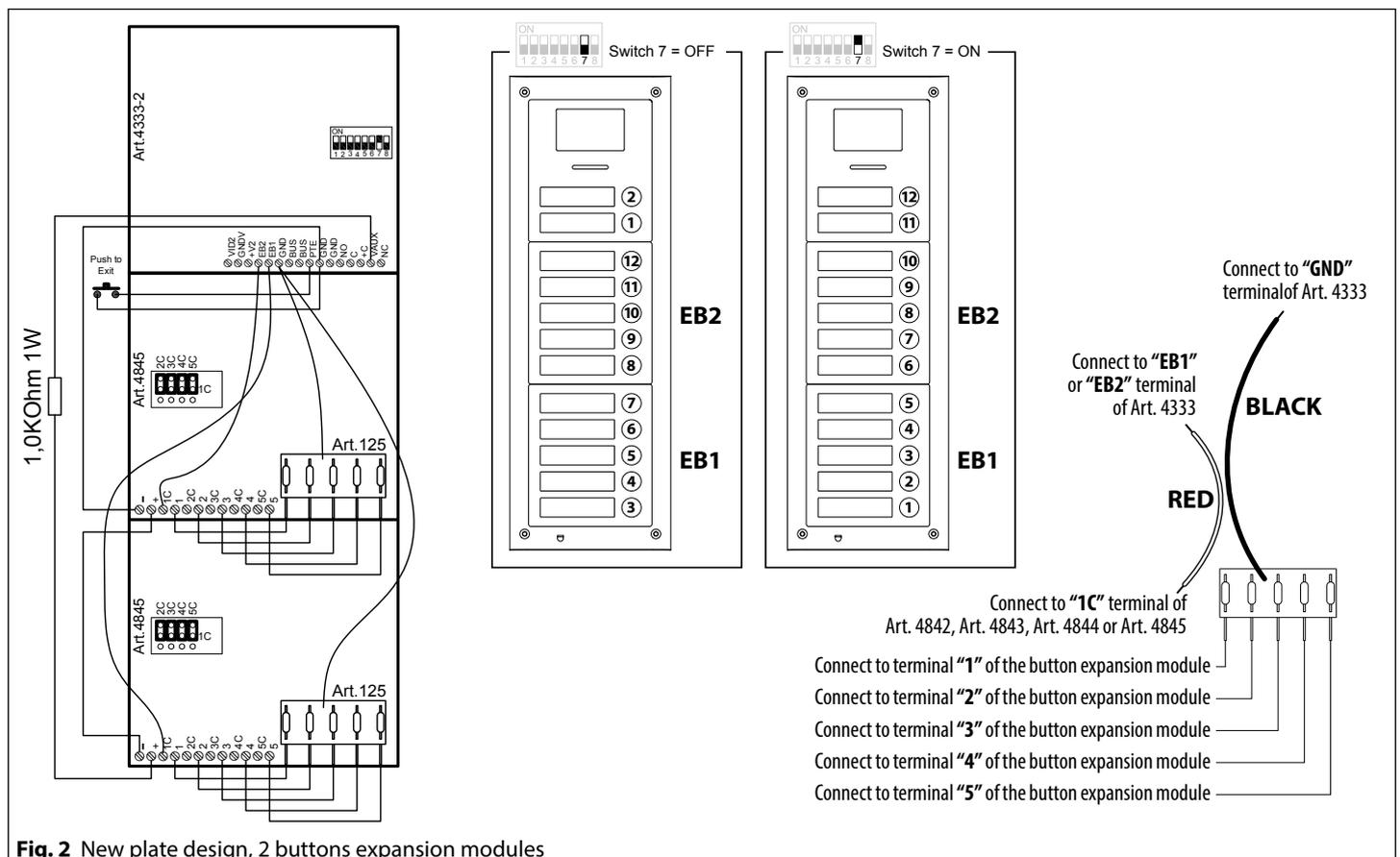
**Fig. 2** New plate design, 2 buttons expansion modules
