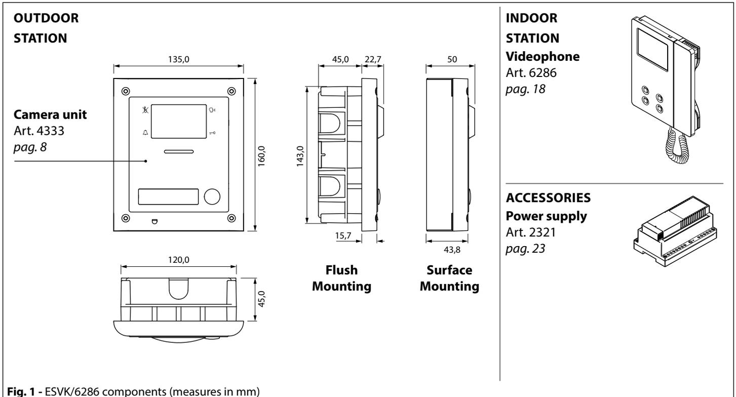
Fig. 1 - ESVK/6286 components (measures in mm)
