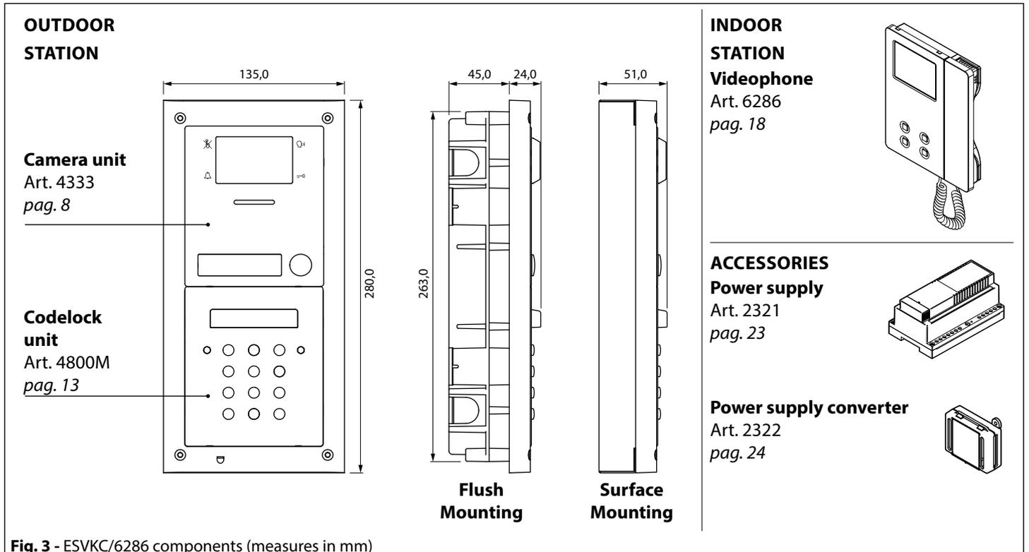
Fig. 3 - ESVKC/6286 components (measures in mm)
