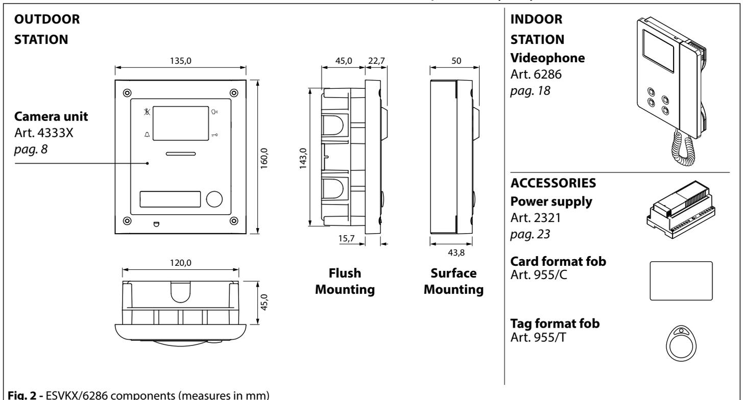
Fig. 2 - ESVKX/6286 components (measures in mm)
