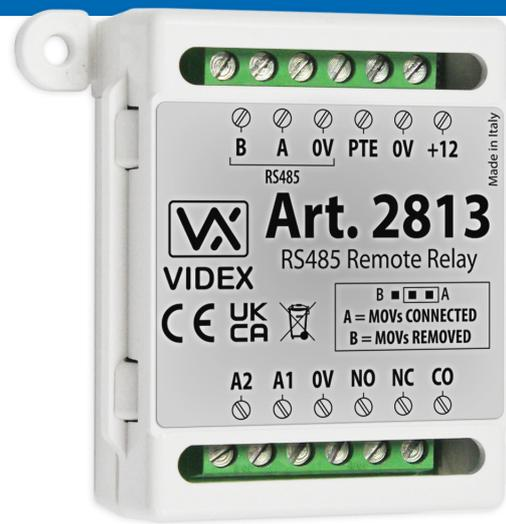
The **Art.2813** is a networkable RS485 remote relay which is compatible with **VIDEX's** 4G GSM intercom modules (excl. **Art.150/4G**) and **VIDEX's** IP system devices.
