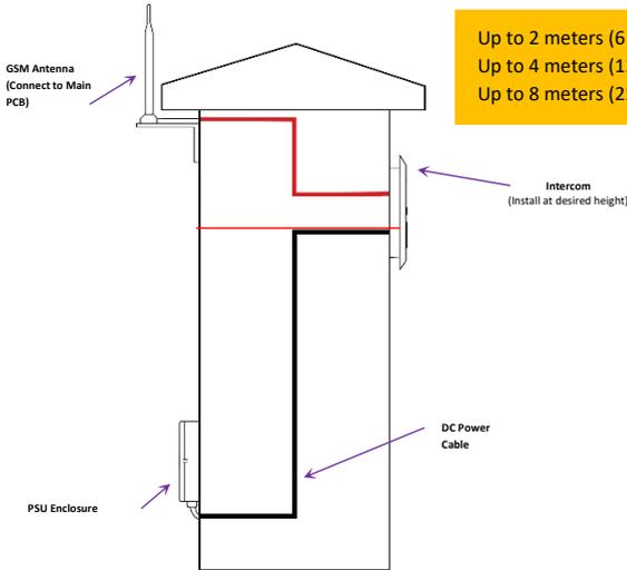
Up to 2 meters (6 feet) use minimum  $0.5\text{mm}^2$  / 18 gauge cable.
