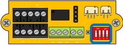
The sounder boards dip switches set the relay number for the auxiliary unit it is in.
