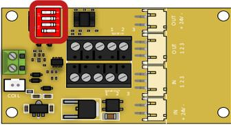
The dip switch of the prox must match the dip switch configuration of the auxiliary it wants to trigger
