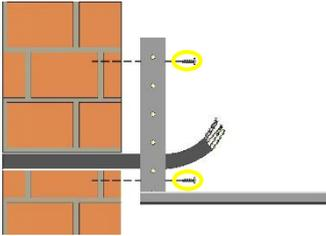
Use the provided mounting holes to attach the intercom via chosen mounting option.
