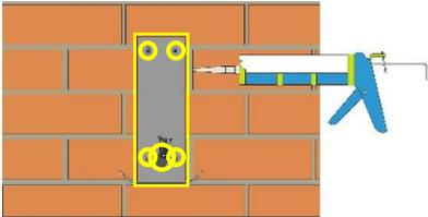
Seal all mounting or cable holes by using sealant such as silicone.
