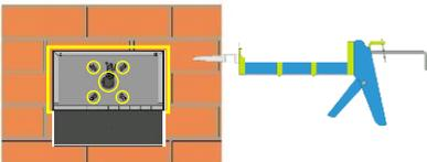
If surface mounting, seal around the back box especially when used on an uneven surface.
