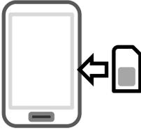
Please ensure the SIM card is a 4G NANO SIM card. Do not use a SIM card for a tablet, as these only support data, and do not support voice and SMS. You simply require a mobile phone type SIM card.
