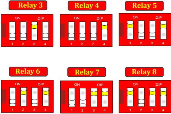
Dip switch configuration for relays 3 to 8 on auxiliary devices.
