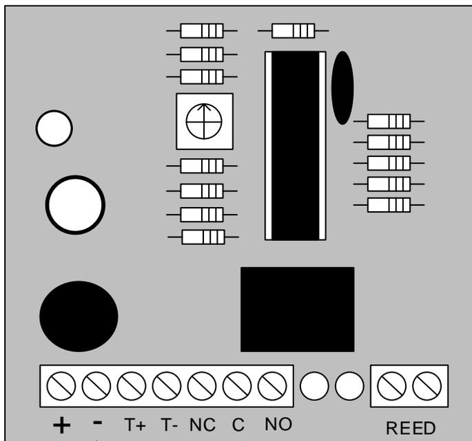
\* Reed: If a door contact is used, once the relay timer has started the timer will reset when it sees the door open and close. This feature prevents the door being insecure for the remainder of the timer period once an entry has been made.
