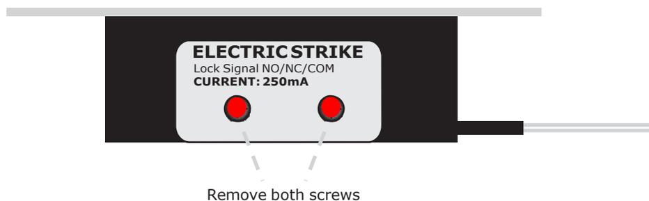
Once the screws have been removed, you will see the two threaded holes on the backplate where the screws were located. To the left of these holes are two more threaded holes, and these need to be lined up to accept the screws being re-fitted.
