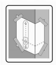
Please note if this unit is a replacement for a Unican 1000 or 5000 series an additional hole will be required to be drilled in the face of door for the code change spindle at the top. The hole in the forend of the door for the latch will also be required to be drilled out to 35mm.
