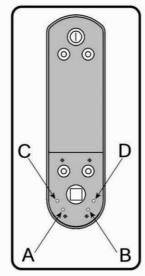
If either of the levers are unable to self return under the spring pressure loosen the grub screw until the lever returns to its horizontal position. If loosening the grub screw does not solve the issue remove one or more of the handle washers until the handle is able to return under its own spring pressure.
