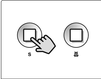
Push the service button **S** to activate the secondary service (if this was set up during the installation). To set up the function of the service button, please contact Videx Technical.
