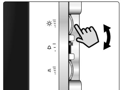
Turn the roller to the right of the brightness control symbol
