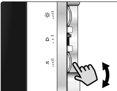
Turn the roller to the right of the speech control symbol
