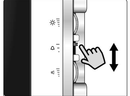
Move the switch, to the right of the call tone symbol
