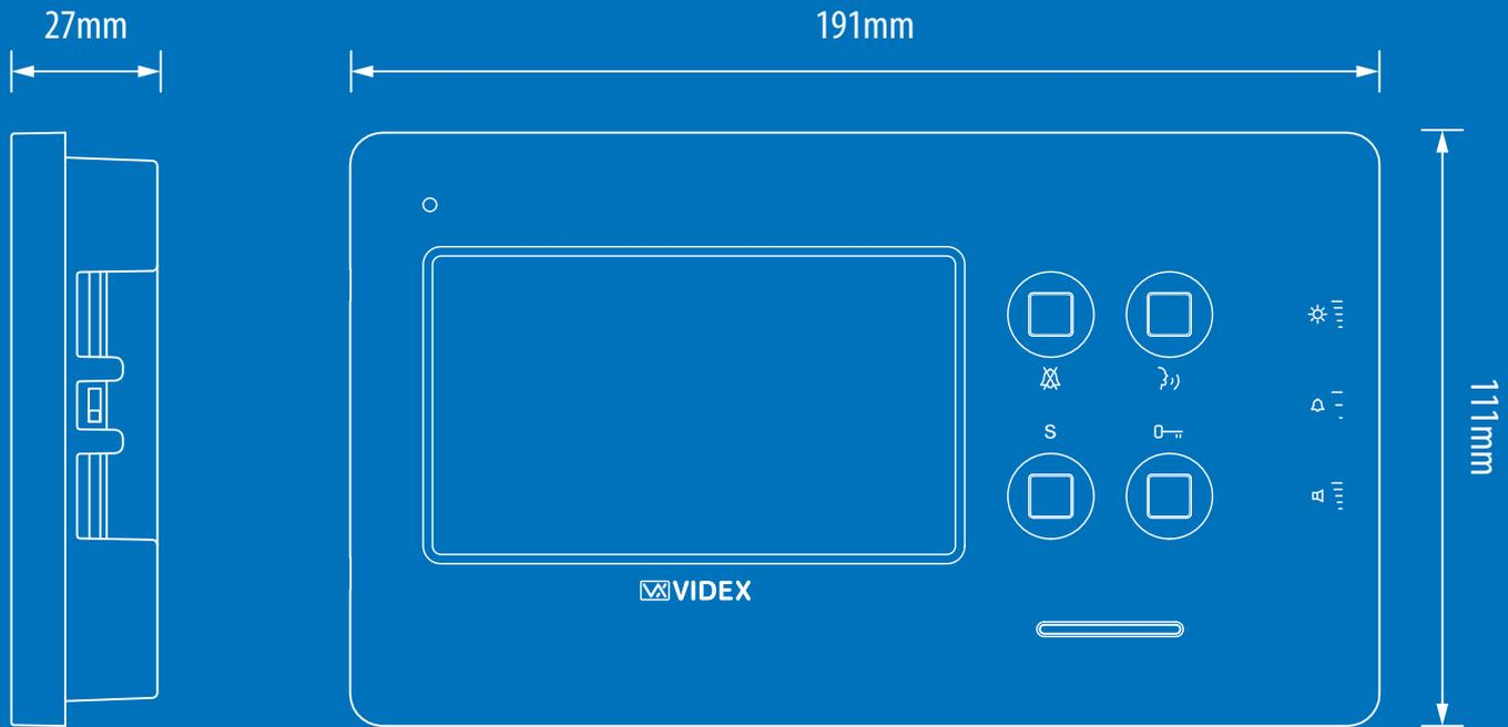
The 6400 series surface mount video monitor with a 4.3" Hi-Res full colour active matrix LCD screen is designed primarily for low and high-rise private developments and individual houses where an attractive and low cost functional videophone is desirable.
