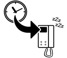
When the conversation time (set up during the installation) has ended, the videophone stops all communication and the system returns to the standby condition.
