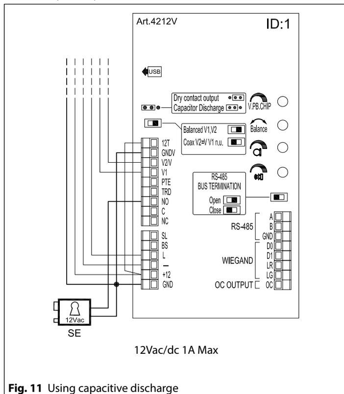
**Fig. 11** Using capacitive discharge
