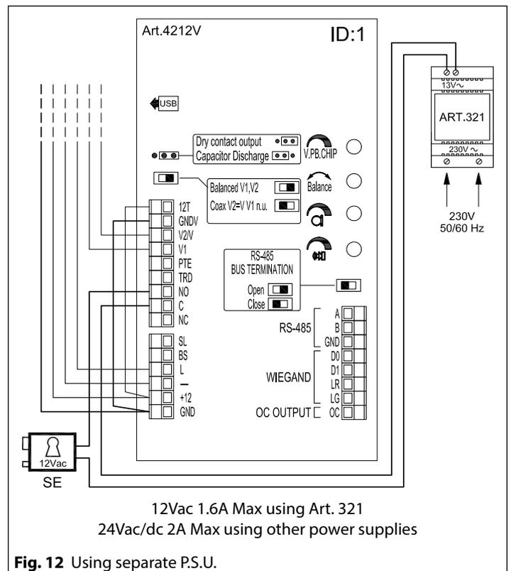
**Fig. 12** Using separate P.S.U.
