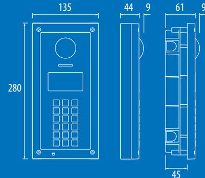
Video panel options include a colour CCD wide angle day/night camera with IR illumination providing a 170° viewing angle as standard.
