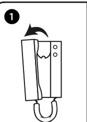
1 Pick up the handset. Press the secondary button as many times as the ID of the BUS relay to enable (if an Art.2305 was setup during the installation, refer to Art.2305 manual).
