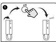
With the handset on the cradle press the lock button 0—π once. The phone will emit a beep, to indicate a call has been placed to the concierge.
