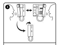
A conversation can begin between the phone and concierge. When the conversation is finished replace the handset back on the cradle.
