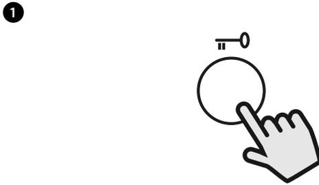
1 During a conversation, with the handset lifted, press the lock button
