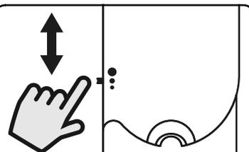
Move the volume switch to the lower position to set the call tone volume to low, to the middle position to set the call tone volume to medium and to the upper position to set the call tone volume to high.
