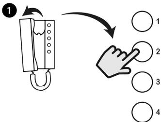
1 Pick up the handset. Press the call button (1 - 4) for the required phone to be called.
