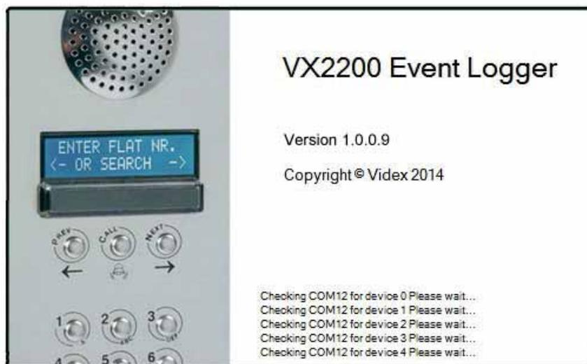
The loading window will appear for a short period as it checks the COM ports of the laptop/PC searching to see if a device is already connected. After the software has checked the COM ports the login window will appear:
