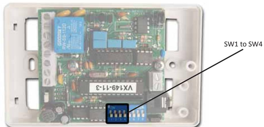
Dip-switches SW5 and SW6 sets up the relay time of the 2214 module.
