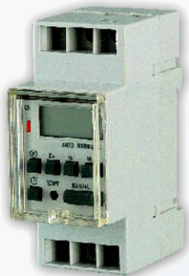
**TH857** is a 7-day, 24 hour digital timer with 6 programmable on/off times each day. Operating at 230Vac, this unit is ideal for providing "free-access" for doors which are electronically locked. The changeover contact is capable of 16Amp switching. An internal battery will store programmed times for up to 200 hours.
