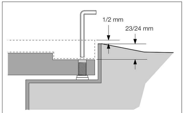
15 - With the treadable flange check the final level with respect to the external floor. If required, using the M16 stainless steel dowels, raise the level and adjust the level positioning.
