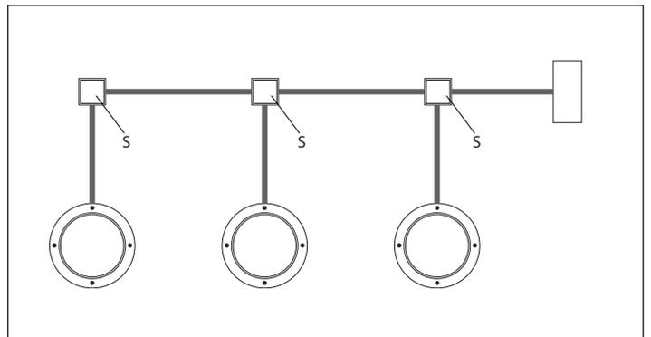
10 -**Attention: The bollard is equipped with a short segment of connection cable equipped with a male IP68 connector. Different size extension cords are available (5 to 25 m), equipped with a female IP68 connector, for connecting to the control unit.** Bring the two parts of the connector together, aligning the arrow with the circle as shown, then fully screw down the fixing nut.
