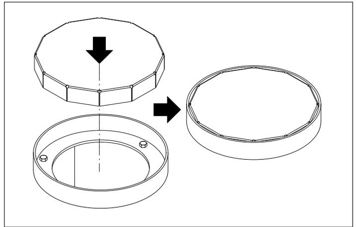
8 - Before inserting the bollard into its housing, remove the previously placed closing or cover making sure that the anchorage housing of the bollard, represented by the grey area, is cleaned carefully. See figures alongside.
