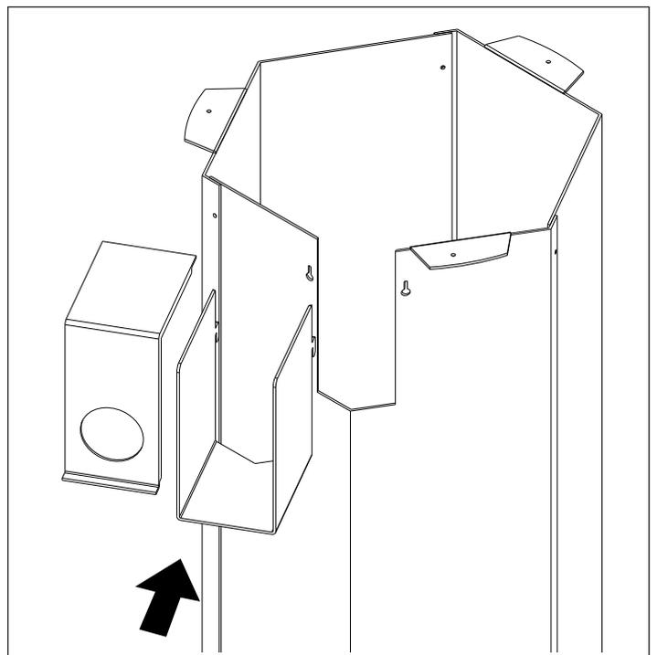
4 - Fix the upper flange using the round head screws provided.
