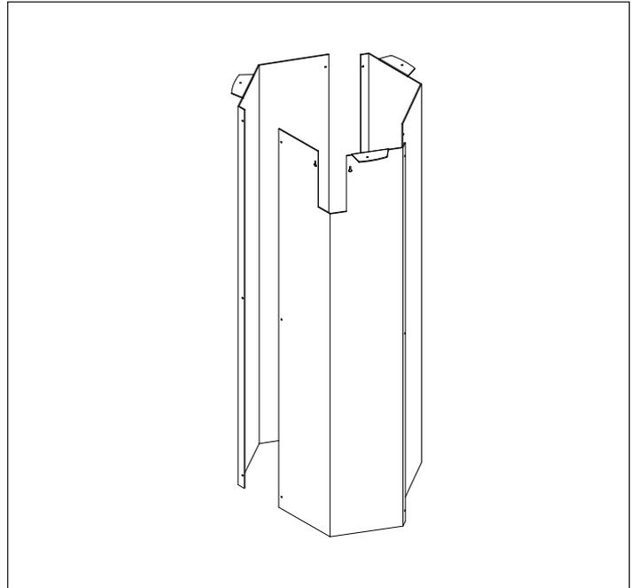
2 - Using the round head screws provided, assemble the hexagonal structure. It is very important to assemble the three elements vertically and on a surface that ensures excellent flatness so as to obtain a reliable support surface for the closing flange. **Attention: The screw head must be placed on the internal side of the foundation case.** See figure alongside.
