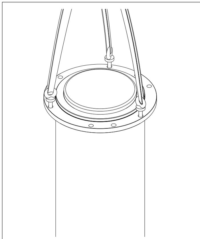
13 - After positioning the bollard inside the case, remove the lifting eye-bolts.
