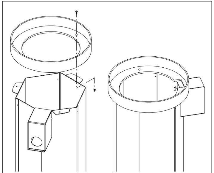
5 - Fit the clamps as in the figure locking them in position with the washer and the M10 hexagonal head screw. Fold them according to the foundation.
