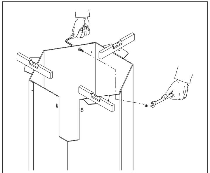
3 - Before fixing the upper flange, insert the metallic protection of the 40 mm diameter corrugated pipe which must be set in the ground to make the subsequent electrical connection with the control unit. See figures alongside.
