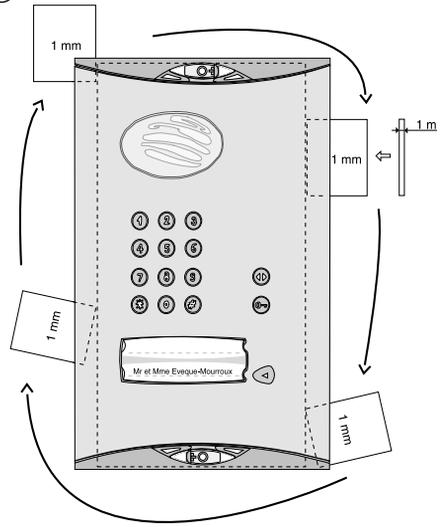
**IMPORTANT:** when the armored cover is positioned on the unit, there should be a 1 mm clearance (use the shim for this purpose) between the pillar and armored cover.
