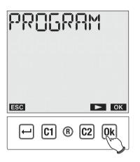
Choose option NEW using keys "C1" and "C2" and press "Ok" to confirm.
