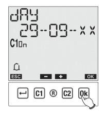
Enter the starting time and duration of the impulse (max 59 seconds).
