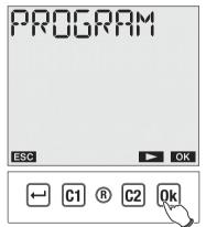
Choose option NEW using keys **"C1"** and **"C2"** and press **"Ok"** to confirm.
