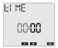
and press **"Ok"** to confirm and go on to the next parameter. The sequence of parameters to be inserted is hours → minutes
