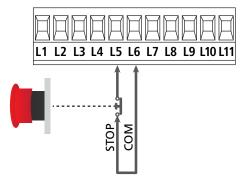
**NOTE:** in case the stop switch is operated while the gate is open, the automatic closing function will always be disabled. To close the gate again, you will need a start command (if the start function in pause is disabled, it will be temporarily enabled to allow the gate release).
