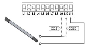
In order to meet the requirements of the EN12978 rules, it is necessary to install safety edges controlled by a control unit continuously checking the proper working. If using control units suited to the test by power outage, connect the power supply cables of the control unit between terminals Z3 and Z2 of the control unit.
