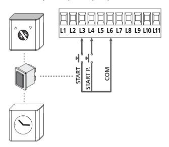
The START function can also be activated by pressing UP key outside the programming menu or by means of a remote control stored on channel 1 (see relevant instructions of MR receiver).
