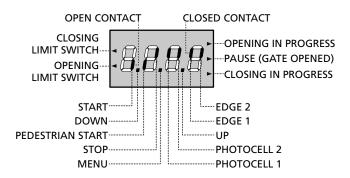
The control panel represents the physical status of the terminal board contacts and of the program mode keys: if the upper vertical segment is on, the contact is closed; if the lower vertical segment is on, the contact is open (the above picture shows an instance where the inputs START, START P, FOTO 1, FOTO 2, COSTA 1, COSTA 2 and STOP have all been correctly connected).
