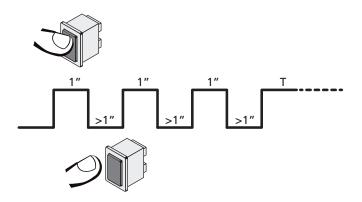
The fourth START command activates the gate in MAN PRESENT mode. To move the gate keep the START command pressed for the duration of the operation (time T). The function will automatically turn off after 10 seconds of inactivity of the gate.
