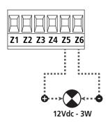
CAUTION: Pay attention to the polarity of the connected device if necessary
