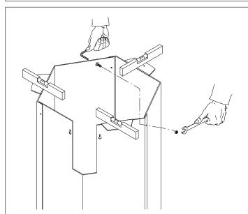
3 - Before fixing the upper flange, insert the metallic protection of the 40 mm diameter corrugated pipe which must be set in the ground to make the subsequent electrical connection with the control unit. See figures alongside.
