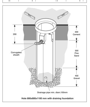
7 - After positioning the case, **make sure that the open recess is covered**, for the entire amount of time that the rising bollard is not inserted, with covering that is suitable to avoid accidents that may involve persons or property. A sheet metal cover is available as an option. See figures alongside.
