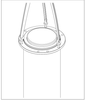
13 - After positioning the bollard inside the case, remove the lifting eyebolts.
