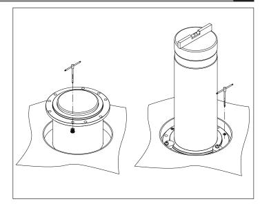
14 - Verify that the distance between the bollard flange and the upper edge of the case/flooring is equal to 23-24 mm.
