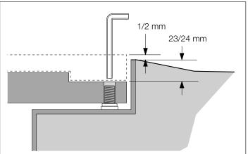
15 - With the treadable flange check the final level with respect to the external floor. If required, using the M16 stainless steel dowels, raise the level and adjust the level positioning. Insert the washers and the M10 hexagonal head screws. Cover the holes with the rubber caps provided. Carry out the electrical connection carefully following the diagram supplied with the control unit. See figures alongside.
