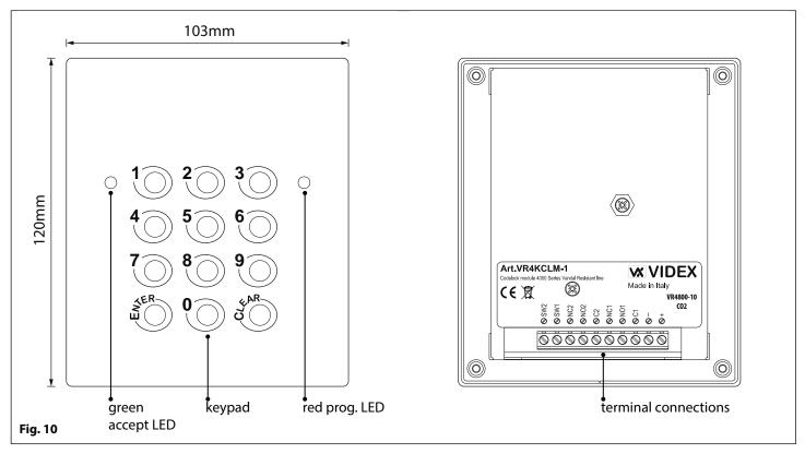
The VR4KCLM-1 codelock module (see **Fig.10**) can be connected to the GSM intercom and is supplied with the GSMVRKC kits. It can be programmed with 2 access codes, one per relay (also see notes on page 10).
