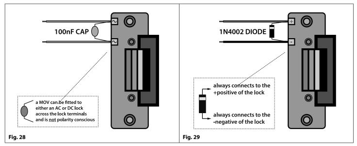
If a 100nF ceramic disc capacitor or a 1N4002 diode are not available then a 14 - 20V MOV (metal oxide varistor) can be fitted across the lock terminals instead (refer to **Fig.28** above) and can be fitted on both an AC and DC lock. Connection examples can also be seen on the wiring diagrams on pages 16 and 23.
