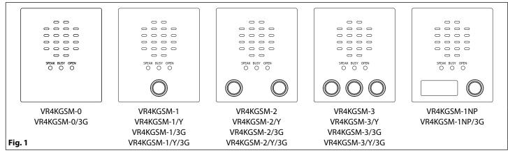
Standard versions of the VR4KGSM modules (e.g. VR4KGSM-0 etc.) works on a 2G network A 3G variant is also available (see Fig.1 above) that works on a 3G network, suffix /3G to the part number as shown.
