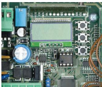
**Built-in receiver**, integrated into the controller, programmable via LCD display.
