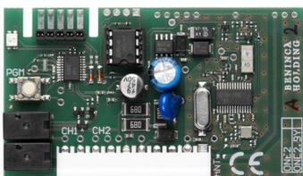
**Plug-in receiver** for controllers equipped with a quick molex connector.
