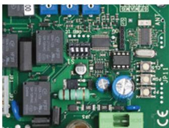
**Built-in receiver**, integrated into the controller, programmable via dip-switches/trimmers.
