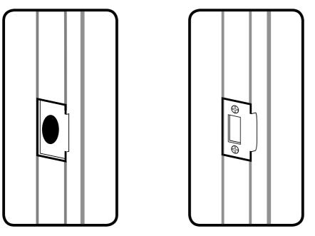
Push the door to the closed position and mark the area on the frame of the door where the strike plate would need to be fitted.
