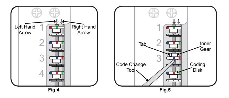
4. Decide what the unit wants to be code to. To change how a button is set in the code – this is done by using a small amount of upwards force lifting the inner gear using the code change tool (part no.12) until the tab on the inner gear becomes visible (as per fig.5).
