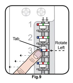
7. Once the first digit has been set, the principle is the same for any other button that you want to set in the code. Once you have programmed all the required digits in your code, turn the handle to reset the coding chamber and ensure that all the buttons that are in the code have the coloured markers in alignment with the left hand arrow on the keypad cover plate. Make sure that any digit that is not in the code has the blue marker of the coding disk in alignment with the left hand arrow.
