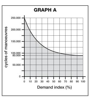
Example of calculation of durability of a Toona series 5 gear motor (refer to Table 2 and Graph A):
