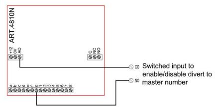
NOTE: WHEN USING THE AO OUTPUT FOR DIVERT TRIGGER IT CAN NOT BE USED AS AN OUTPUT FOR ANYTHING ELSE.
