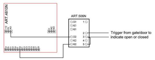
NOTE: WHEN USING THE AO OUTPUT FOR STATUS INDICATION IT CAN NOT BE USED AS AN OUTPUT FOR ANYTHING ELSE.
