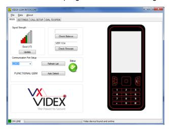
When the program loads, it checks all available ports for the GSM unit. If found, the GSM unit goes online with the PC. From the main screen it is possible to:-
